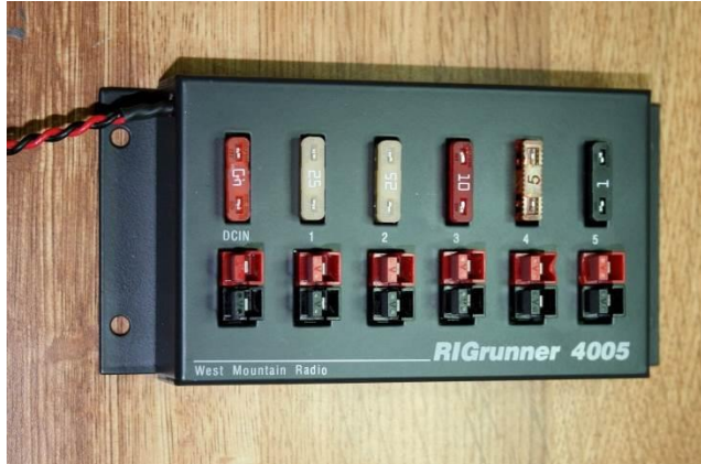
Rigrunner 4005 Note: 5V DC regulator added to provide external DC for USB Hub
