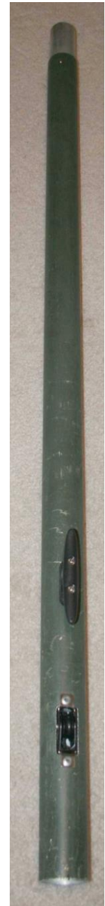
Bottom mast section with halyard pulley and cleat.
