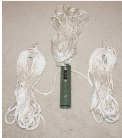
Top Hat with guy ropes and halyard pulley
