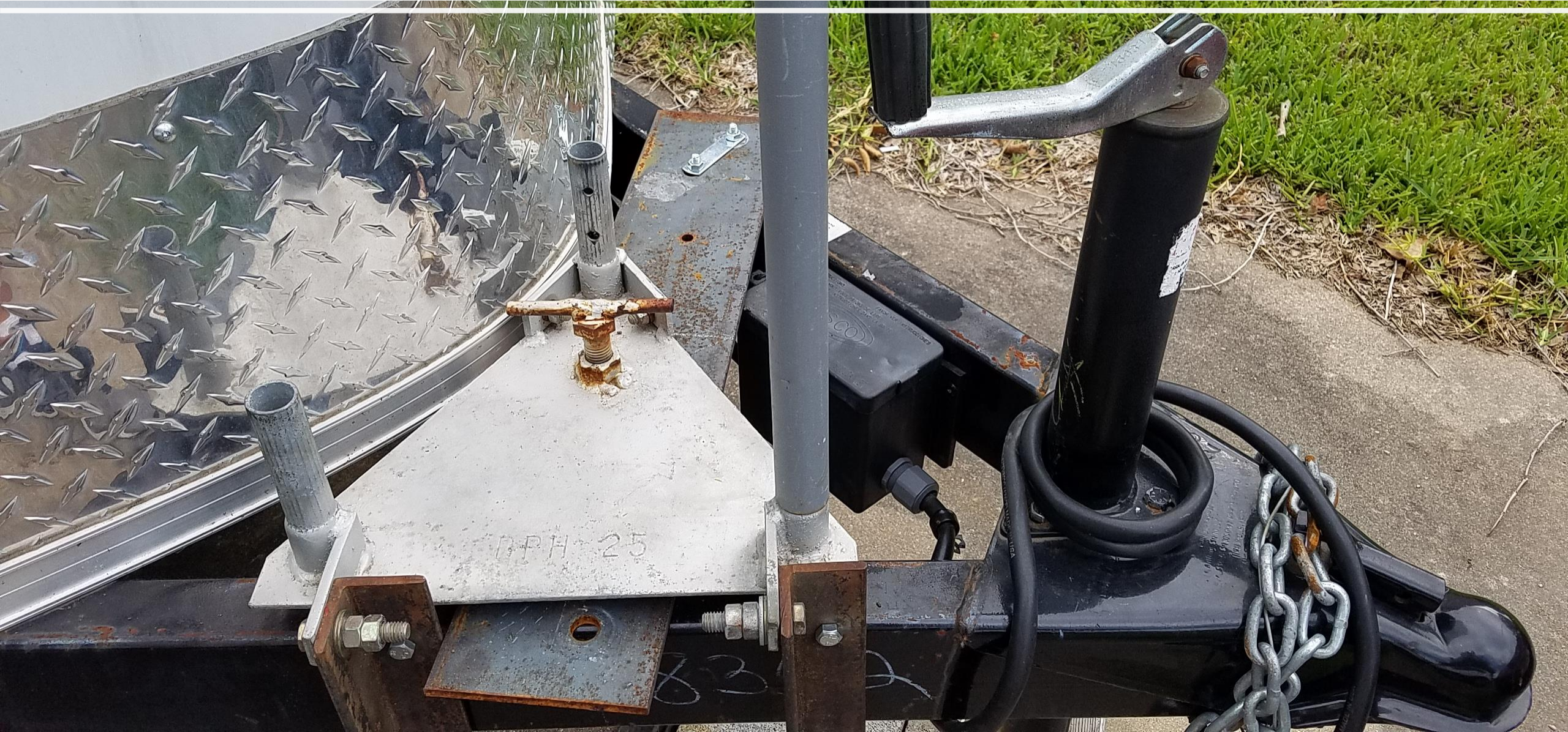
Rohn 25G hinge base mounted on trailer nose
